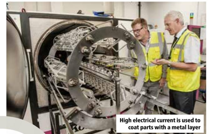
High electrical current is used to coat parts with a metal layer
